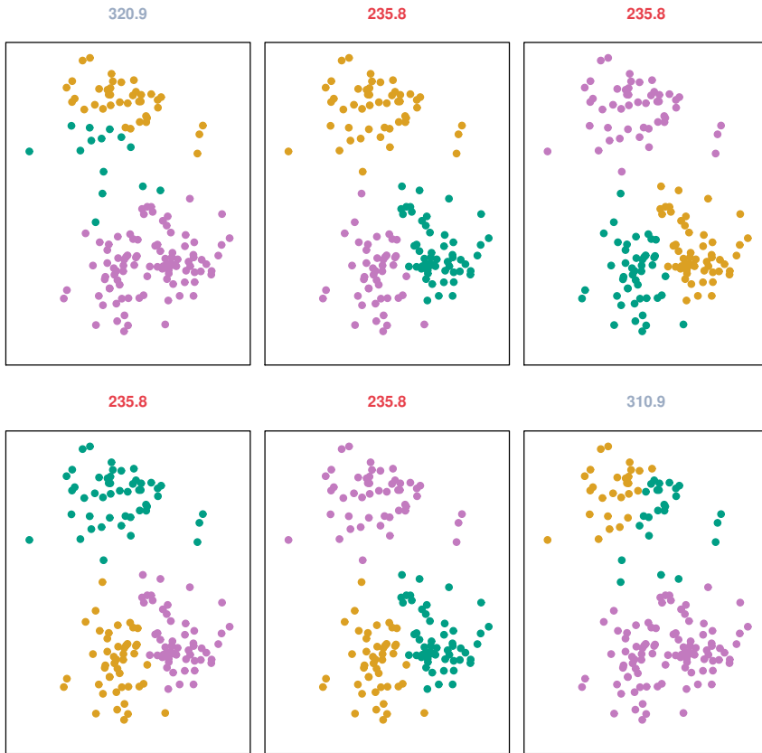
FIGURE 12.9. K -means clustering performed six times on the data from Figure 12.7 with K = 3 , each time with a different random assignment of the observations in Step 1 of the K -means algorithm. Above each plot is the value of the objective (12.17). Three different local optima were obtained, one of which resulted in a smaller value of the objective and provides better separation between the clusters. Those labeled in red all achieved the same best solution, with an objective value of 235.8.
